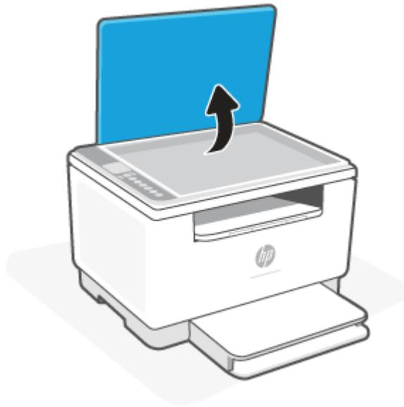
2. Load your original print-side down and align it with the marking on the rear left corner of the glass.
