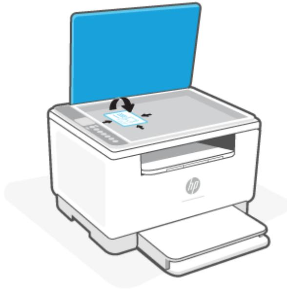
4. Close the scanner lid and press
