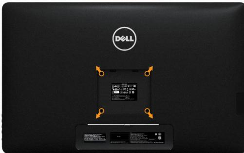
**NOTE:** For use only with UL-listed wall-mount bracket with minimum weight/load bearing capacity of 7.11 kg.
