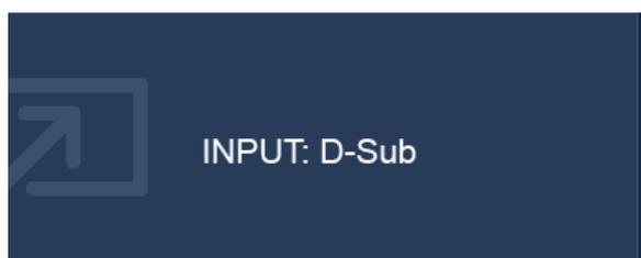
Press the **ENTER** key to toggle between different PC video signal inputs that may be connected to your monitor. The setting will take effect immediately. See also [Input on page 35](#).
