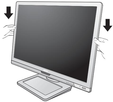
⚠️ Avoid placing hands near the bottom of the monitor stand as the descending stand might cause personal injuries. Keep children out of reach of the monitor while performing this operation.
