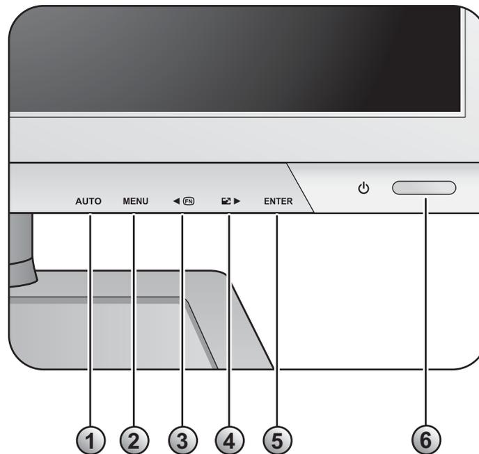
1. **AUTO**: Adjusts vertical position, phase, horizontal position and pixel clock automatically.
