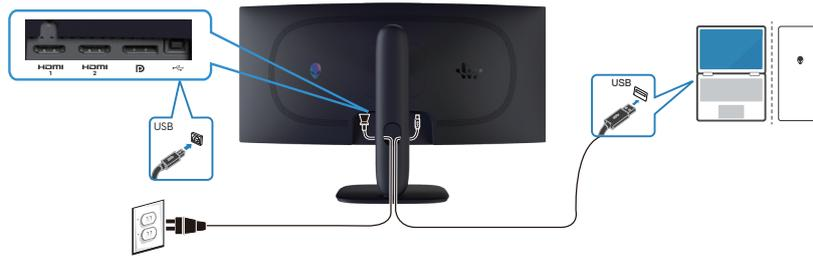
**Figure 24. Connecting the USB Type-B (Type-B to Type-A) cable**
