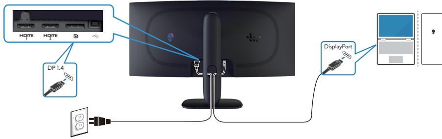
**Figure 22. Connecting the DisplayPort (DP to DP) cable**
