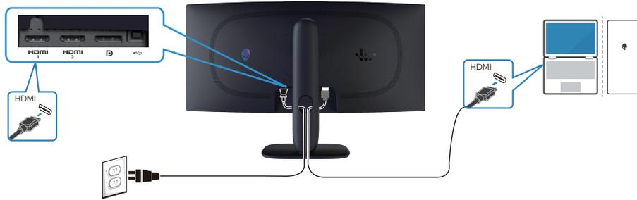
**Figure 23. Connecting the HDMI cable**
