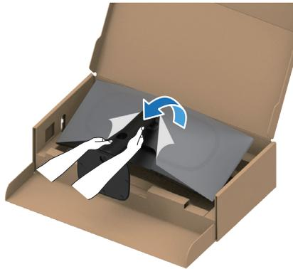
**Figure 16. Hold the stand riser and lift the monitor**
