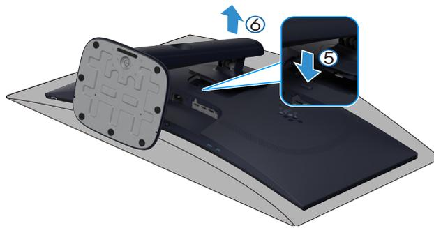
**Figure 26. Removing the monitor stand**
