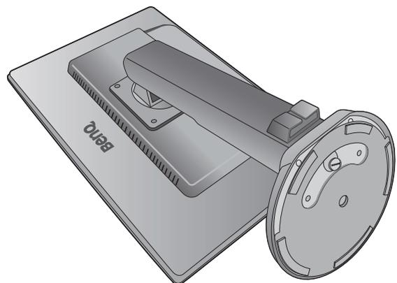
Extend the monitor to the maximum extended position. Then tilt the monitor. And rotate the monitor 90 degrees counterclockwise as illustrated.
