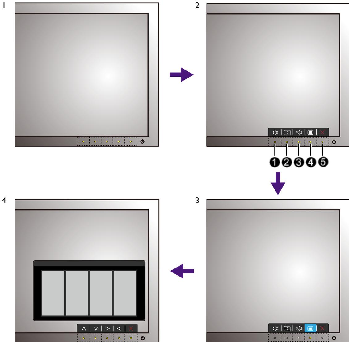
1. Press any of the control keys. Alternatively, press the **OK** key on the OSD Controller.
