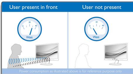
PowerSensor is a built-in 'people sensor' that transmits and receives harmless infrared signals to determine if the user is present and then automatically reduces monitor brightness when the user steps away from the desk, cutting energy costs by up to 80 percent and prolonging monitor life
