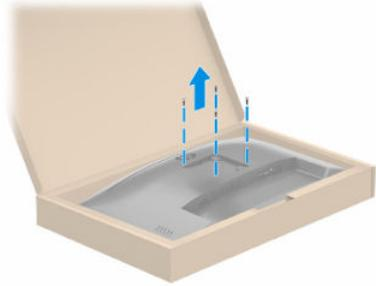
2. To attach the monitor head to a swing arm or other mounting device, insert four mounting screws through the holes on the mounting device and into the VESA screw holes on the back of the monitor head.
