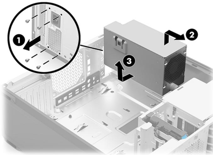
Reverse this procedure to install the power supply.
