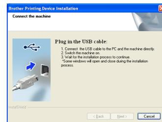
**e** Connect the USB cable to the USB port marked with the
