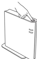
This feature will automatically detect which mode (WPS or AOSS™) your wireless access point/router uses to configure your machine.
