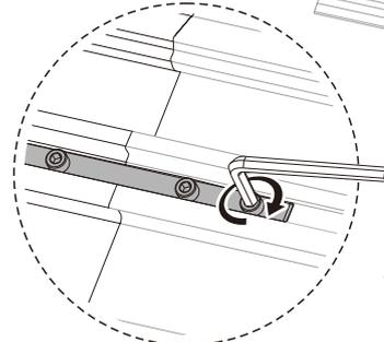
Using the joining piece connect additional ductings as required.
