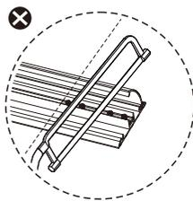
Using a hacksaw cut the ducting to desired length
