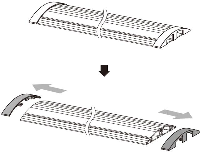
Remove the plastic end caps on each side of the ducting.
