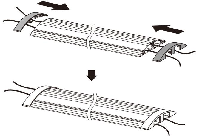
Re-attach the plastic end caps on each side of the ducting.
