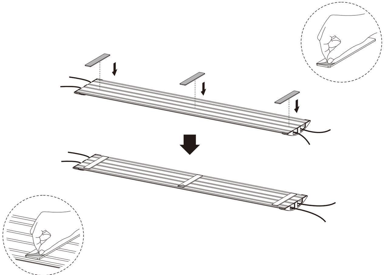
To prevent the ducting from moving, attach double-sided tape as required.
