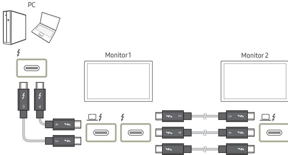
Dual display (daisy chain) support depends on your PC and the connected Thunderbolt™ 3 / 4 cable. The Thunderbolt™ 3 port on your PC must support dual 4 K @ 60 Hz output, and the particular 40Gbps Thunderbolt™ 3 / 4 cable (⚡⚡, ⚡⚡) need to be purchased separately. For detailed specification of the Thunderbolt™ 3 / 4 cable, visit the official Thunderbolt website.
