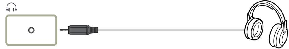
— The headphones or earphones jack supports only the 3 conductor tip-ring-sleeve (TRS) type.
