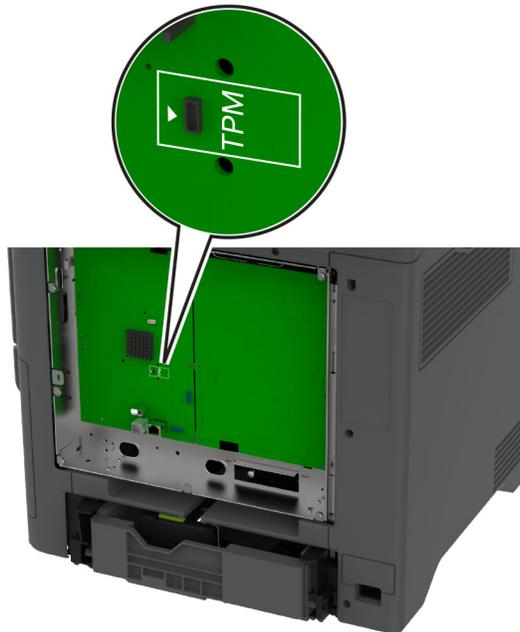
5 Attach the module to the TPM connector.
