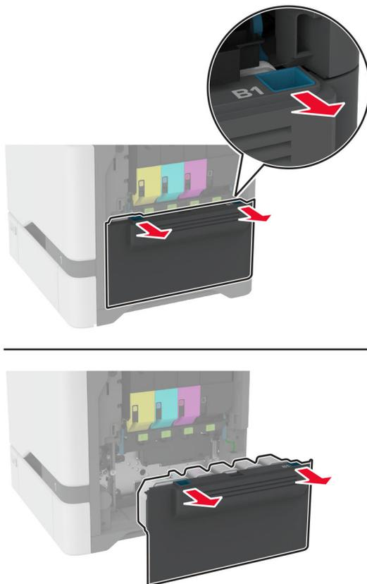
**Note:** To avoid spilling the toner, place the bottle in an upright position.
