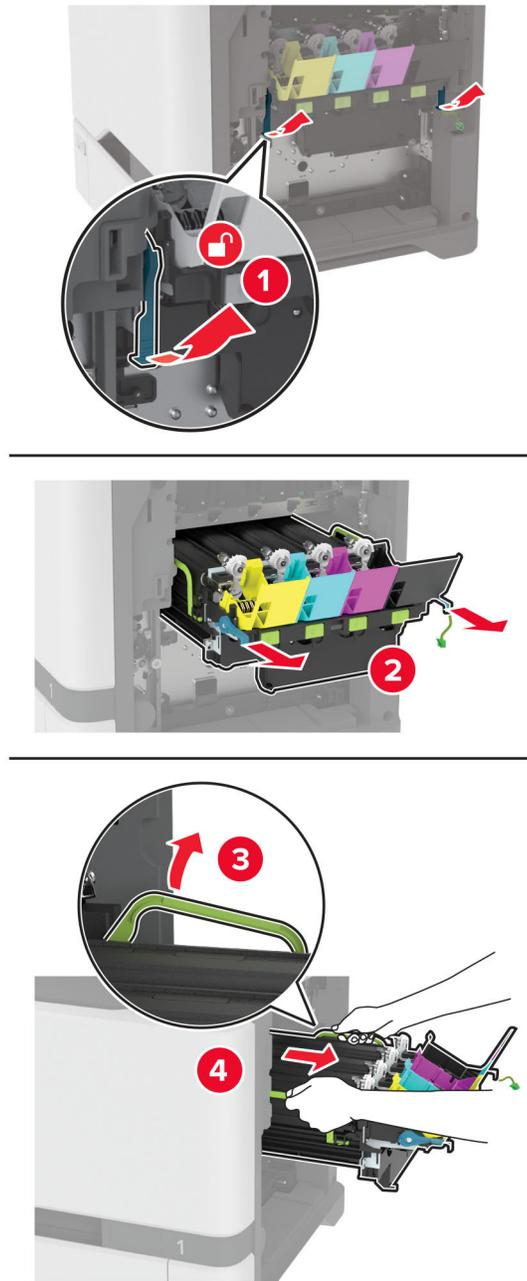
**Note:** To avoid scratching the imaging kit or damaging the photoconductor drum, place the imaging kit in an uplifted position.
