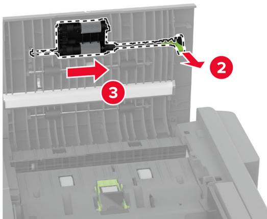
**3** Remove the used ADF separator roller.
