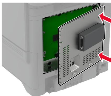
7 Attach the controller board shield.
