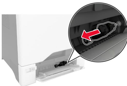
**4** Apply isopropyl alcohol to a soft, lint-free cloth, and then wipe the pick roller.
