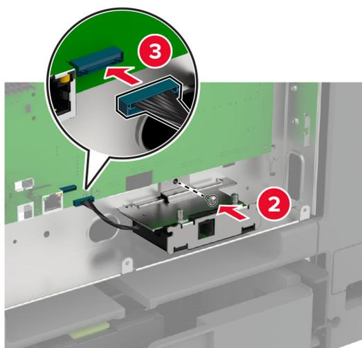
**7** Attach the controller board shield.
