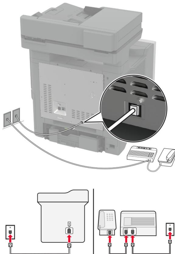
**1** Connect one end of the telephone cable to the line port of the printer.
