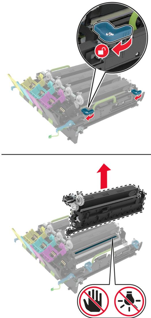
**Warning—Potential Damage:** Do not expose the photoconductor unit to direct light for more than 10 minutes. Extended exposure to light may cause print quality problems.
