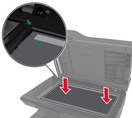
**Note:** Make sure that the scanner glass pad is aligned correctly on the edges of the scanner glass.
