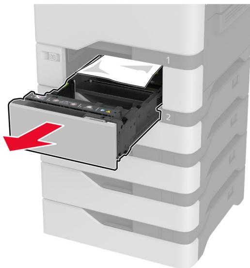
**Warning—Potential Damage:** A sensor inside the optional tray is easily damaged by static electricity. Touch a metal surface before removing the jammed paper in the tray.
