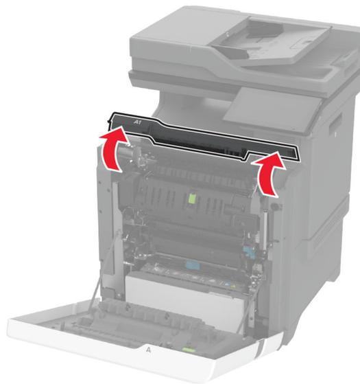
**3** Remove the used fuser.
