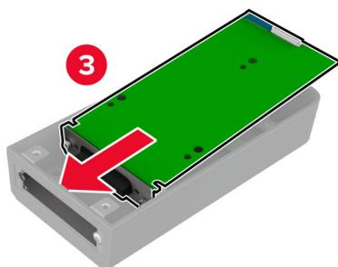
5 Attach the housing to the controller board shield.
