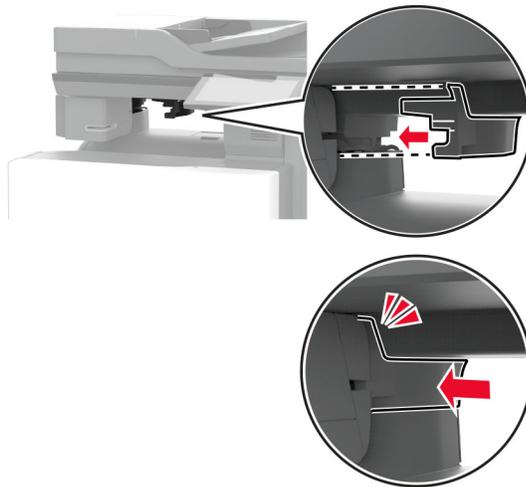
**Note:** Make sure that the power supply is secured.
