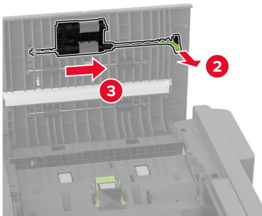
**3** Remove the ADF separator roller.
