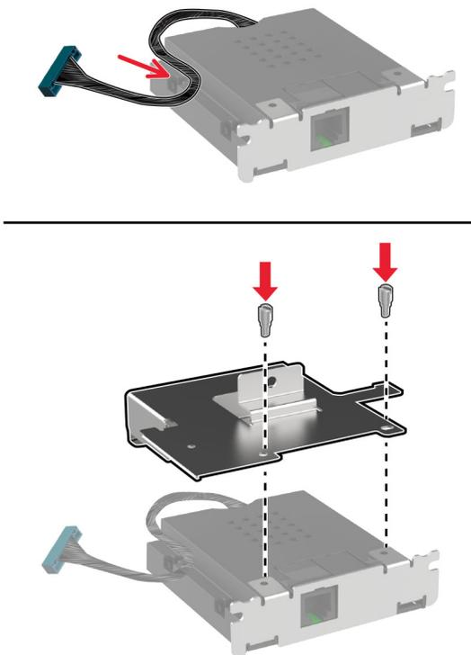
**6** Install the fax card and attach the connector to the controller board.
