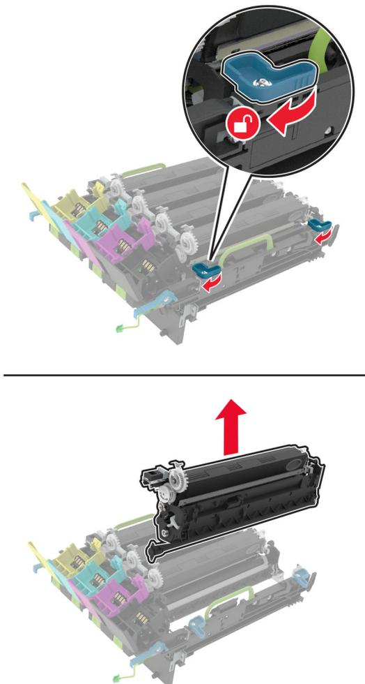
**Warning—Potential Damage:** Do not expose the photoconductor unit to direct light for more than 10 minutes. Extended exposure to light may cause print quality problems.
