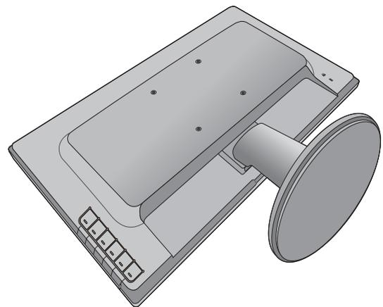
Insert a pointed object such as a screwdriver to the hole above the monitor stand arm, and then push the screwdriver against the release button inside the hole. Then pull the monitor stand backward away from the monitor.
