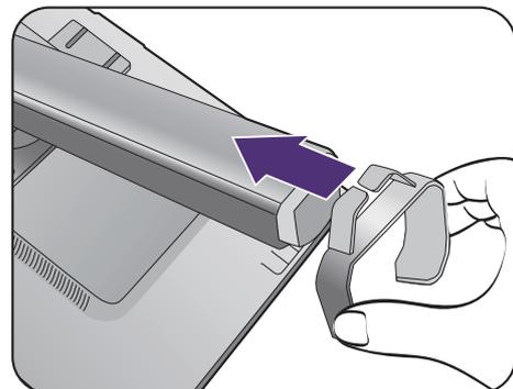
Orient and align the stand base socket with the end of the stand arm, then push them together.
